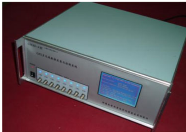
Figure 21. GPS multiple-antenna switching device [64].
