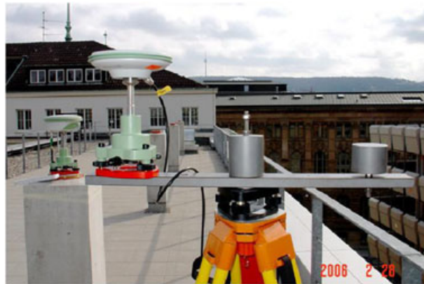
Figure 14. Rover Antenna mounted on a tripod provided with a rotating arm [29].
