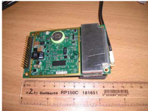
Figure 8. The JNS100 OEM board GPS receiver [23].
