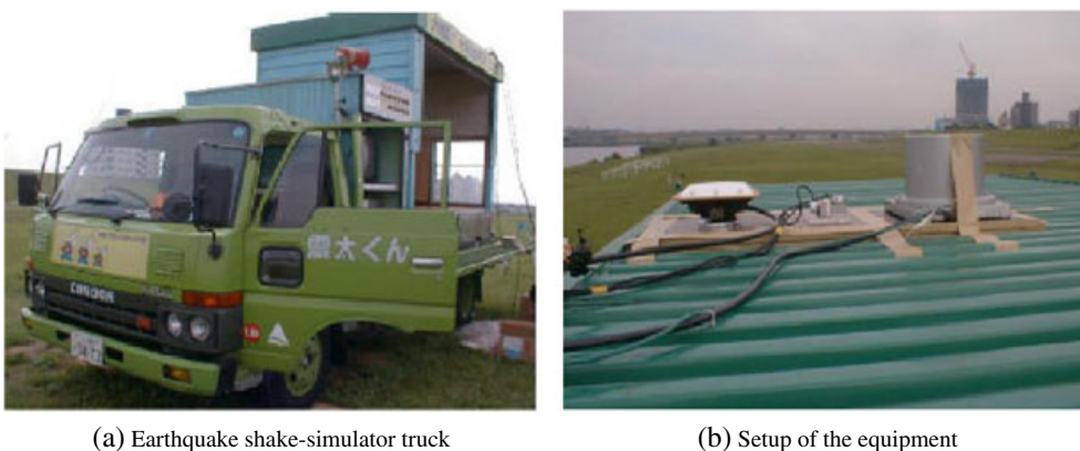
Figure 3. GPS seismometer experiment [18].
