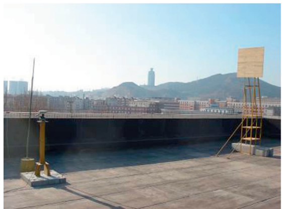
Fig. 12. Set-up of the reflector at different distances of antenna.
